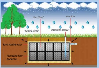
**VersiTank®** units enveloped with a filter fabric, allows rainwater to percolate through the filter into the tank below whilst ensuring that solids, including mud and clay are filtered and prevented from entering the tank.
