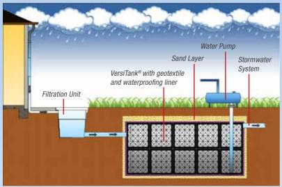
**VersiTank®** units installed with an impermeable shell membrane, enables filtered rainwater channeled via pipes or allowed to slowly percolate into the tank from the surface to be retained and stored.
