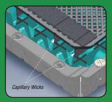
Placement of Planting Media The MEP® Tray has a fitted Support Plate for placement of a geotextile filter. Its small apertures stop excess planting media from getting into the reservoir.
