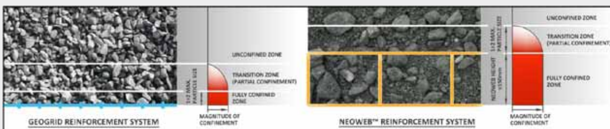
Comparison of Geogrid vs Neoweb Confinement Zone
